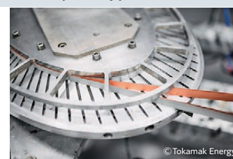
© Tokamak Energy Manufacture of ST-80 magnet coils
